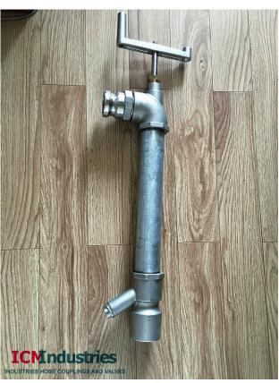
1. The updated fittings have platform for the automatic Actuator, making the automatic snow making easier. No more fixed support.
