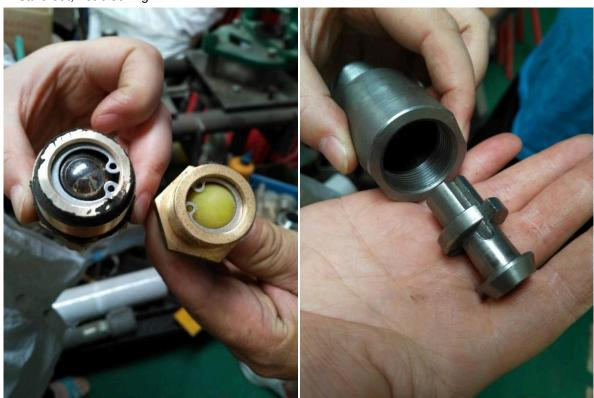
4. Change the bronze drain valve body to stainless steel 304 material. That is because the bronze stem seat fitting always pulled thread, but stainless steel valve body have better performance on this item.
